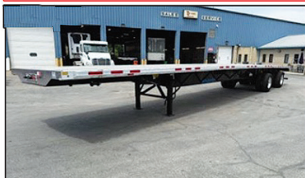
NEW WABASH COMBO W/REAR AXLE SLIDE, 53'x102", Alum Floor, Winch Track Both Sides, Cal Legal, Alum Outer Wheels, $35,950 Plus FET
