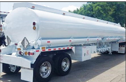
(4) 2014 HEIL PETROLEUM TANKS, 9200 Gal., 3200/2300/1100//2600, Trough Bottoms, One Double B/H, Air EV's, Civacon Top & Bottom Probes, Air Ride, $52,000
