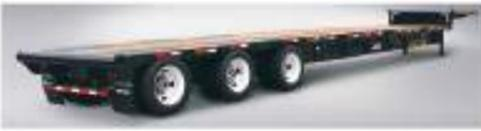
New Transcraft Dropdeck 53'x102 Tridems, with 8 5/8" Live Tail Roller, Pin Pockets, round pipe at transition, sliding winches.
