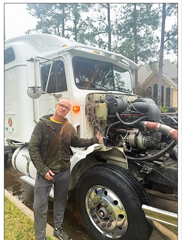
Todd from Houston, Texas is running a 1999 IH 9400 with a Cummins N14 Celect with a HT-60 Switchblade Turbocharger.
