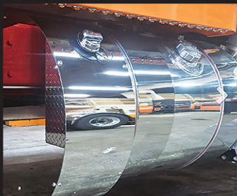
DEF Tank Covers
